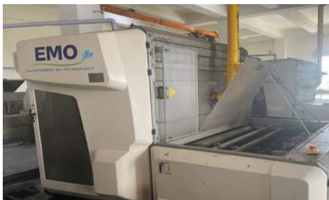
Cleaning of Filter Cloth in Sludge Dewatering Machine
